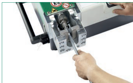
Tooling head for cutting ring assembly based on settings manually defined by the operator
